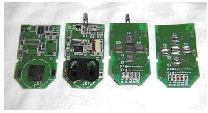
area where the keypad targets were. For applications requiring high reliability, the keypad targets should be gold plated.
